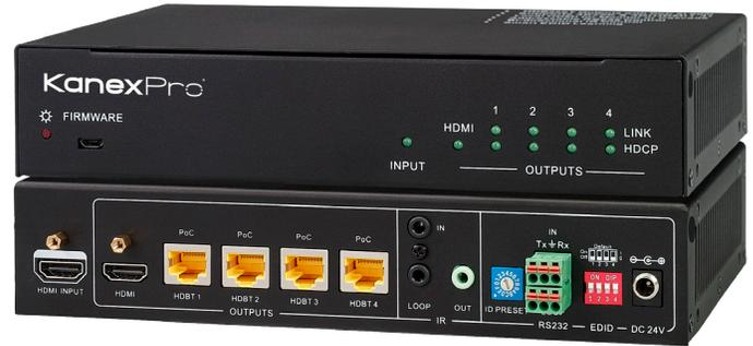
The KanexPro HDMI 1X4 Splitter over HDBaseT is a half-rack width distribution amplifier, which reliably distributes one HDMI source signal to four Ultra HD 4K displays over single CAT6. It can also be daisy-chained to support up to 8-displays without losing any signal integrity using HDBaseT technology.
